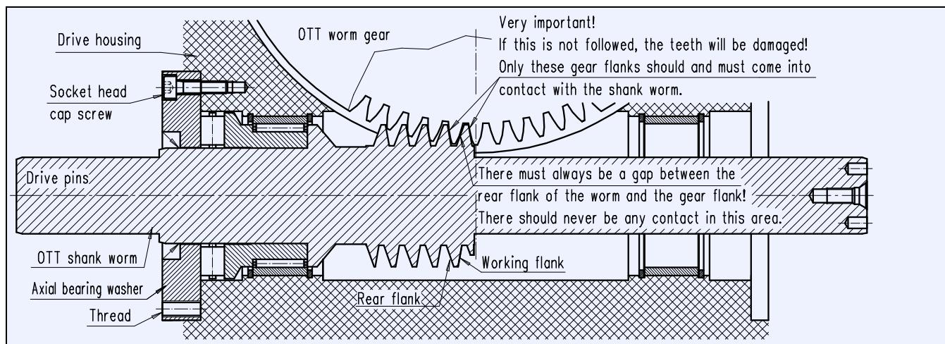
5.) Lubricate working flank of shank worm.
