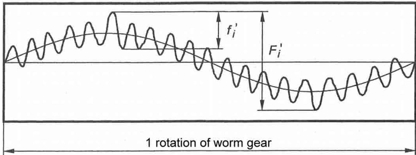
$F_i'$  = Tangential composite error (largest rotation error within one worm gear revolution)
