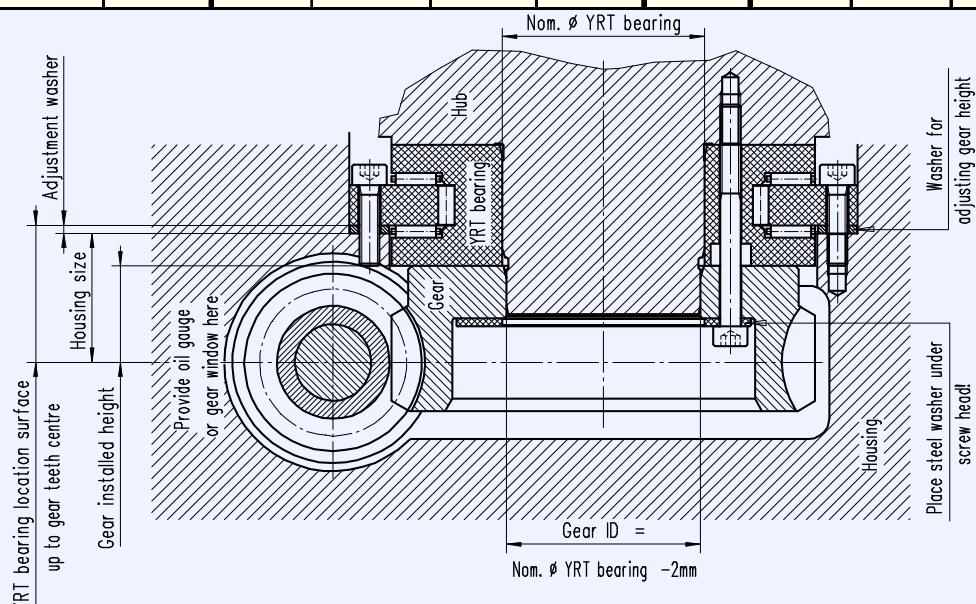
**Gear housing - required internal contour**
