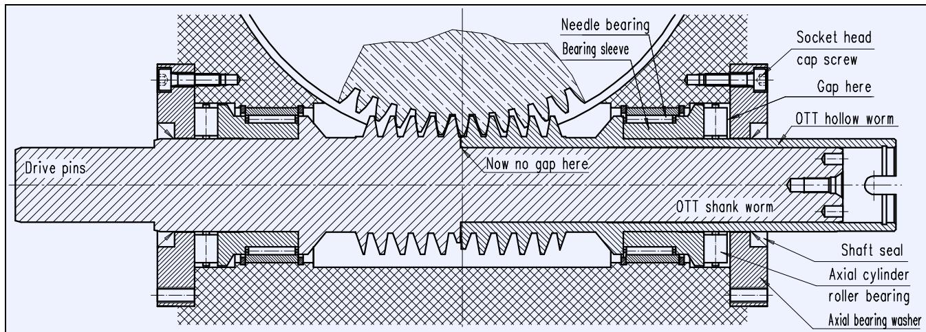
13.) Place hollow worm on shank worm, and press shank worm on to gear flank. **Do not draw in!**
