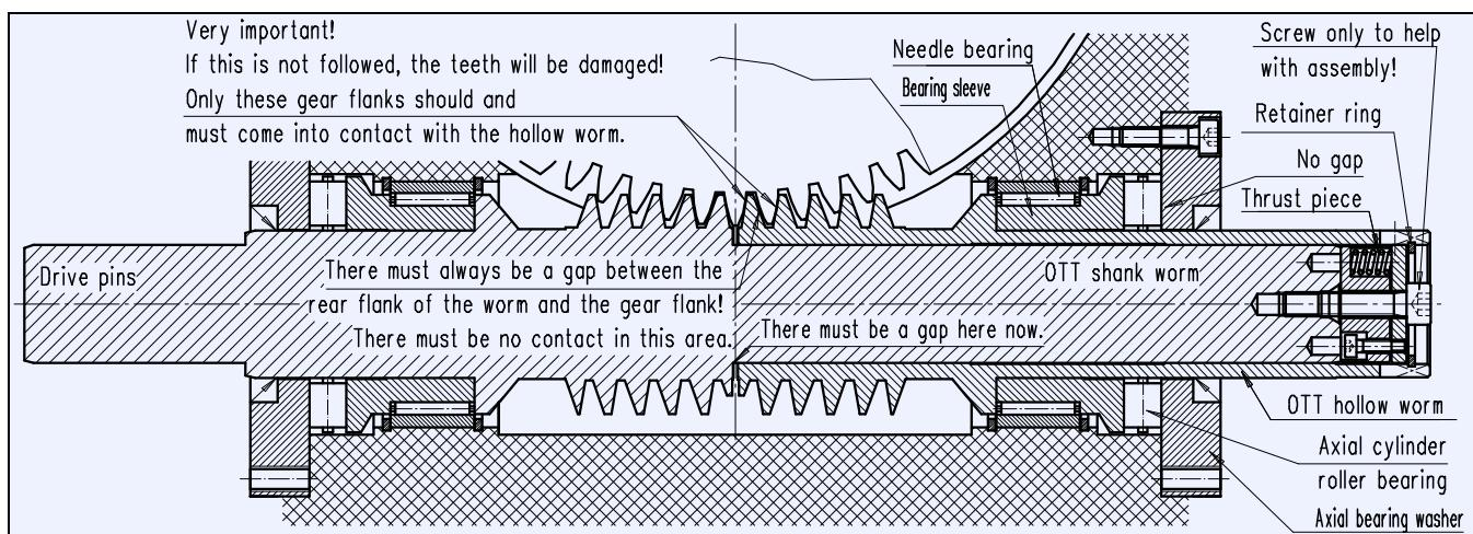
16.) Hold the shank worm firmly and turn the hollow worm in the opposite direction to slide the worm halves against the working flank. There will be an even clearance of the flanks and axial bearing. There will now be a gap between the shank worm and the hollow worm.
